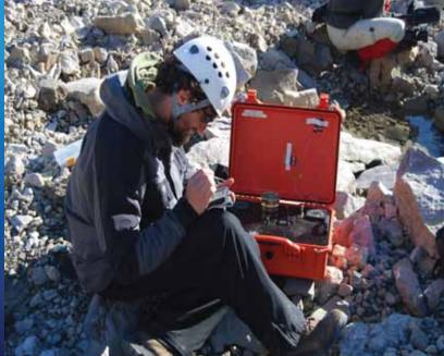
Self contained X-ray Diffraction / X-ray Fluorescence instrument
